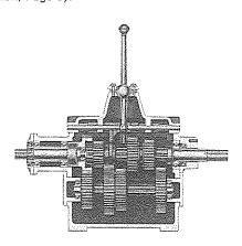
SECTIONAL VIEW OF FOUR-SPEED SELECTIVE TRANSMISSION. Gears are 1" face, machine generated and heat treated. The spline shaft is heat treated tool steel. Ball bearings are used throughout.
