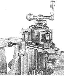
DUAL FEED MECHANISM with cover removed. This mechanical feed mechanism has a double square thread feed screw which rotates in bronze bearings in the upright. It is simple, rugged and so nearly automatic that astounding cutting speeds and blade life are realized even though an inexperienced operator may seldom change feed settings, regardless of the varying sizes and types of steel he may cut. (Refer to detailed explanation, Page 3).
