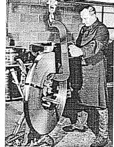
Coil being loaded on a stock reel. Hook is easily removed from the coil after releasing the hoist.
