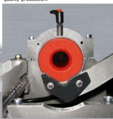
Using field-proven principles, the Quick Six guides bar stock through a single guide tube without scratching the bar stock when loading. Pressurized hydrostatic oil film is used to absorb vibration and friction. This quick change guide tube properly supports the bar to assure high spindle speeds
