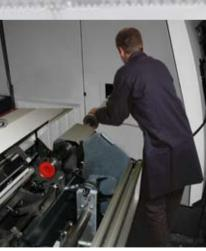
The Quick Six offers an easy-to-slide Z-axis retraction. It frees access to the spindle for changing spindle liners or for lathe maintenance operations. The chassis retracts up to 19" on the upper part of the stands and maintains perfect alignment with the spindle. This mechanism saves time spent in realignment.
