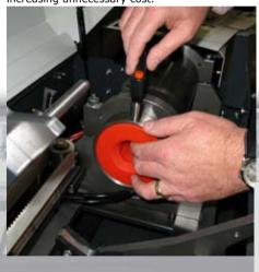
The Quick six offers the industry's widest range for a 6-foot automatic magazine bar loader accepting 1/2" to 3-1/8" diameter bar stock. Changing the single guide tube is quick and easy. When changing diameter simply follow the prompts on the remote control to enter the bar diameter, part length and guide tube ID. The Quick Six does the rest in record time.
